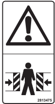
6 WARNING! Articulation area Nobody is allowed stay within the unsecured articulation area.
