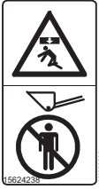
10 WARNING! Do not walk under raised lifting arms. Stay at a safe distance from the machine.
