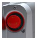
If sudden danger occurs, the system can be shut down by pressing the emergency stop button on the front of the Powerbox. This action can also be performed by a third person. It is therefore important to always set up the Powerbox at some distance from the work area.
