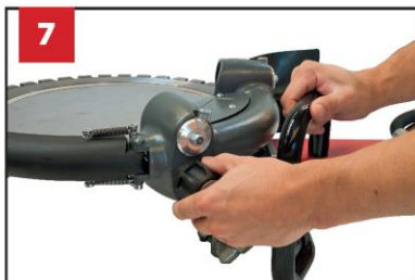
Adjust the guide roller against the drive wheel - turn the black knob clockwise until it stops. Both guide rollers should be equally tightened! NB: It cannot be overtightened
