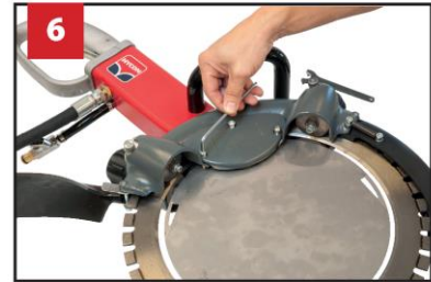
Mount the water blade and the cover.
