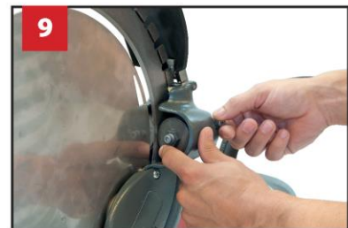
If the support roller is correctly adjusted you can turn the roller by the finger. If it cannot turn it is too tight.
