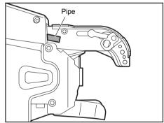
Align the groove of wire guide B attached to arm B with the pipe, and assemble arm B.
