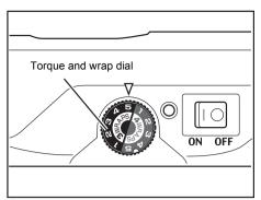
② This dial allows you to set 3 wraps / tie or 4 wraps / tie and also you can adjust the torque.
