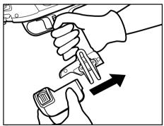
Mount the battery pack on the tool's main body until a click is heard. Turn the Main Switch ON
