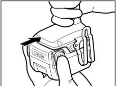
3 Insert the charged battery pack into the tool until a click is heard.
