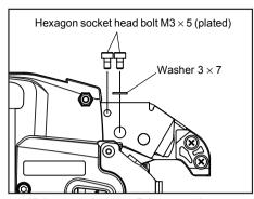
Make sure that arm B is securely assembled and tighten the 2 (plated) hexagon socket head bolts M3 × 5. (Tightening torque: 15.2lbF·inch (172cN·m))
