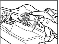
3 Regularly clean the feeding mechanism In order to maintain the performance of the tool, periodically clean up the mechanism around the feed gear. Using the Air Duster or like, blow the dust and the iron sand off around the feed gear.
