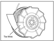
Peel off the tape fixing Tie-Wire by about 2" (5cm). Stretch out the tip of the wound Tie-Wire.
