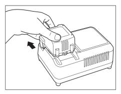
After you have recharged the battery pack, remove it from the charger.
