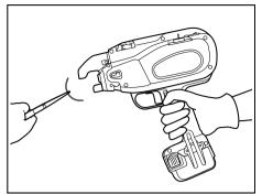
① Tool feeds the wire about 6" (150 mm) and cuts the wire automatically.Remove the cut end of the wire with pliers.
