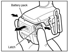
When charging the Battery pack, remove it by pushing on its latches from both sides while firmly holding the grip of the tool.
