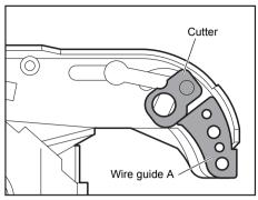
5. Fit the cutter and assemble wire guide A.
