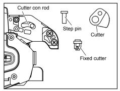
Remove the cutter and the fixed cutter, and clean them. (The removable parts are the cutter, fixed cutter and step pin.)
