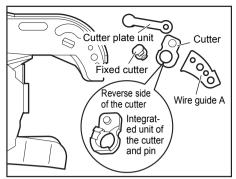
Remove the cutter and the fixed cutter, and clean them. (The removable parts are the cutter, fixed cutter, wire guide A and cutter plate unit.)
