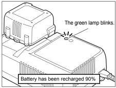
When the battery pack has been recharged, the "red" lamp turns off and the "green" lamp blinks.
