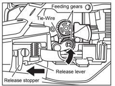
Release the release stopper, and confirm that the release lever has returned to its original position and that the feeding gears are clamping the Tie-Wire. This completes the Tie-Wire mounting operation.
