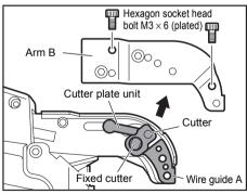
2. Remove arm B and the 2 (plated) hexagon socket head bolts M3 × 6.
