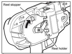
3 Push the reel stopper to release the reel holder.
