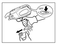
① Be sure to turn the main switch OFF, to lock the trigger and detach the battery pack.
