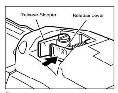
Press the release lever, and confirm that the release lever is caught in the release stopper.
