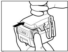
Mount the battery pack on the tool's main body insert the charged battery pack on to the main unit until a click is heard.
