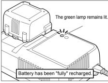
You can use the battery pack when quick charging is complete. However, if you leave the battery pack on the charger, recharging will continue. When the battery is fully recharged (to 100% capacity), the "green" LED lamp lights up (and a long beep sounds for approximately 2 seconds).
