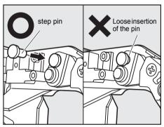
4. Insert the step pin into the hole and then into the connecting rod hole.
