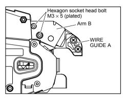
1. Loosen the 2 (plated) hexagon socket head bolts M3 × 5.
