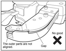
Make sure that arm B is securely assembled and tighten the 2 (plated) hexagon socket head bolts M3 × 6. (Tightening torque: 15.2lbF·inch (172cN·m))
