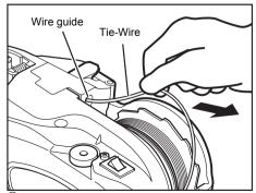
Remove the Tie-Wire from the wire guide.
