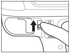
Pull to the left slightly and upwards to UNLOCK.
