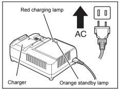
② Plug the charger into a wall socket (120V). The red light, a current-carrying indicator, will flash on and off with two short (Pipi) beep sounds
