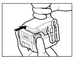
③ Insert the charged battery pack into the tool until a click is heard.
