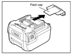
A Pack cap that is used to prevent short circuits must be removed from the terminal of the Battery pack.
