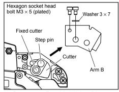
2. Remove arm B and the 2 (plated) hexagon socket head bolts M3  $\times$  5.
