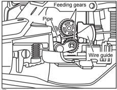
Insert the tip of the stretched out Tie-Wire into the Wire Guide. Then put it into the Pipe.
