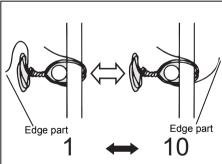
② The feed dial is a mechanism to adjust feed rate of the Tie-Wire. When the edge part length is not appropriate after binding, use this dial to adjust it.
