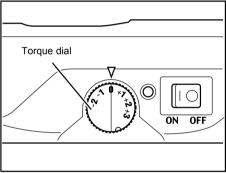
2 This dial allows you to adjust wire tension torque slightly.
