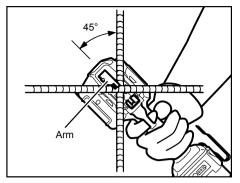
1 Tilt the tool 45° angle to the crossed re-bars.
