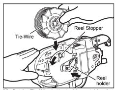
Set the Tie-Wire in the tool by matching the side of the Tie-Wire as shown in the picture. Then slide the Reel stopper so that the Reel Holder can be pushed in the Reel. Then push the Reel Holder and fix it by sliding the Reel stopper.
