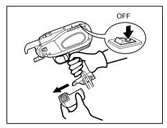
Be sure to turn the Main switch OFF, to lock the Trigger and detach the Battery pack.
