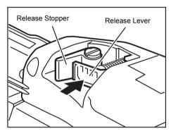
Terest the Release Lever of this equipment, and confirm that the Release Lever is caught in the Release Stopper.
