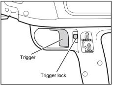
1 Unlock the Trigger before using the tool.
