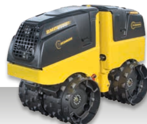
BMP 8500 Operating weight: 1,595 kg Centrifugal force: 72/36 kN Working width: 610 mm / 850 mm
