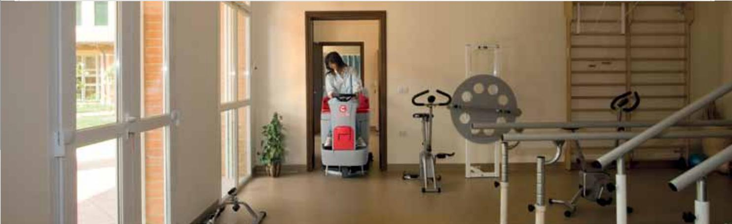
Innova 60 B is a battery ride-on scrubbing machine with automatic traction drive available in the version with 1 disc brush, with a working width of 61 cm.
