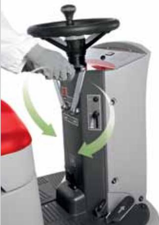
The brush head and the squeegee are lowered/raised by simply using two levers
