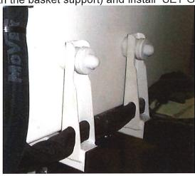
G.2 Once the bottom insulation pieces have been put, it will not be possible to install "SET G.1". Install "SET G.2" as shown in this diagram.
